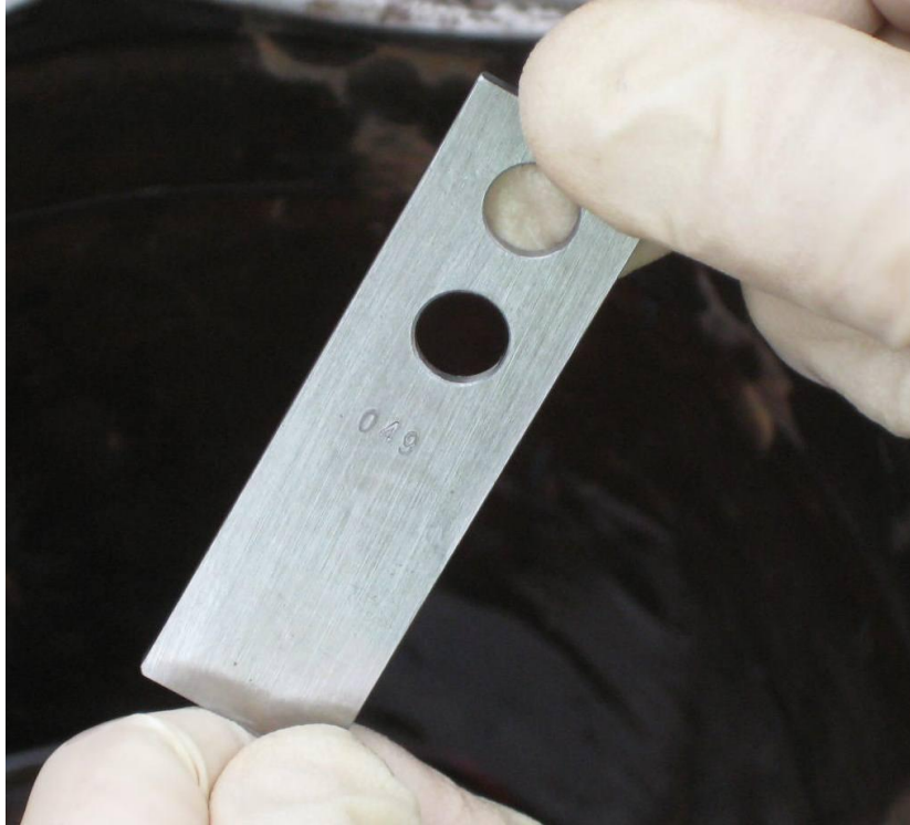
New steel corrosion coupon
