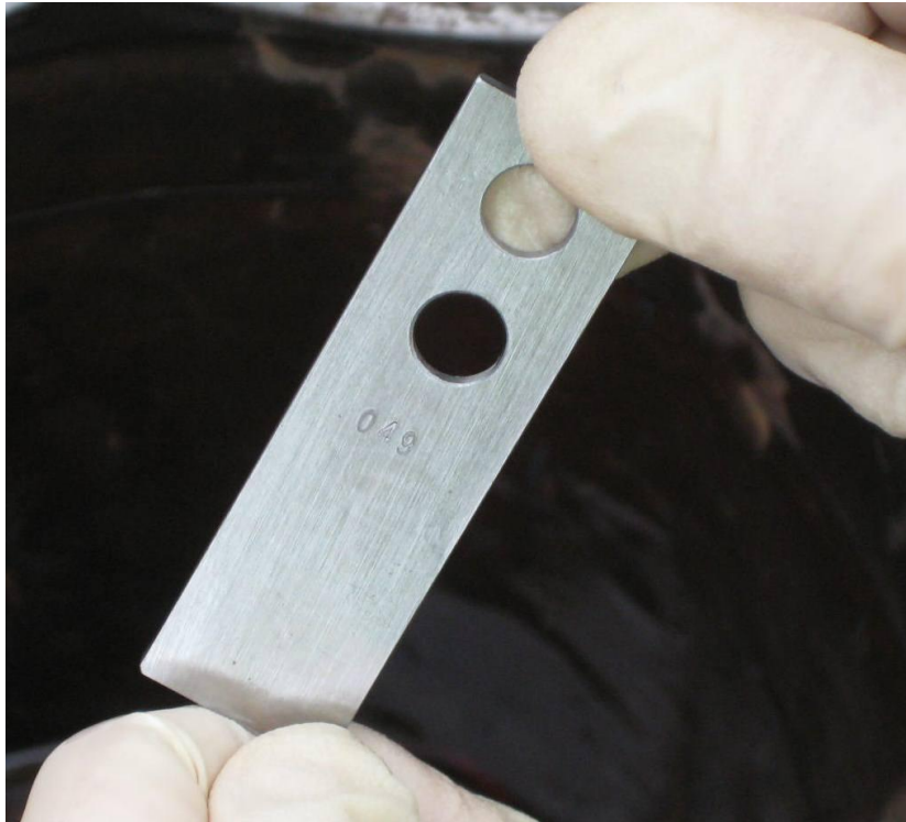
New steel corrosion coupon
