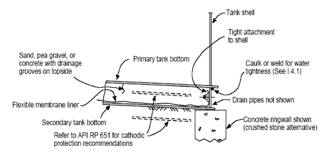
Figure I-4—Double Steel Bottom with Leak Detection at the Tank Perimeter (Typical Arrangement)
