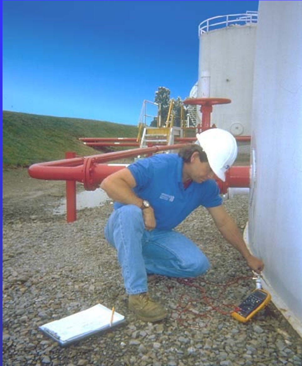
Annual Cathodic Protection Survey
